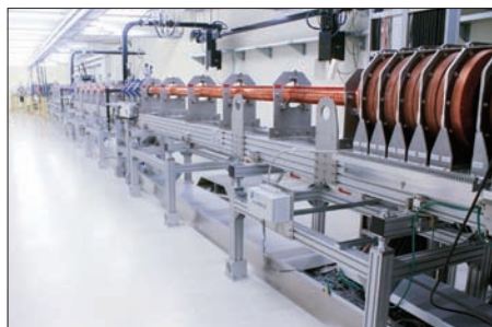
The linac system for the TPS, with the gun and bunching sections.
